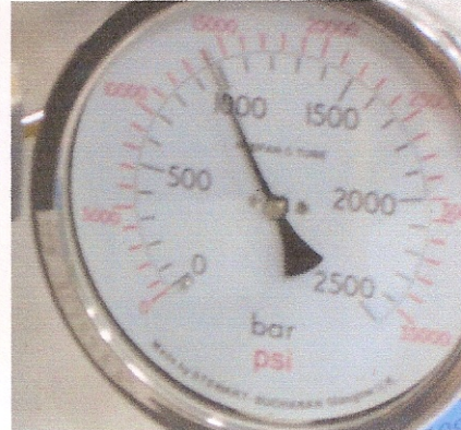
Fig.8) Approx. Burst Pressure
